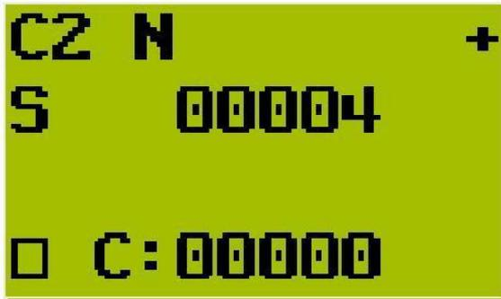
A cursor flashes to change the parameter. Select with the arrow keys the parameter "S" and press "OK". Change with the arrow keys the parameter "S" and verify your selection with "OK". To cancel the procedure press "ESC".
